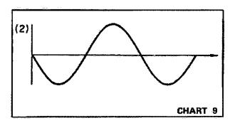
2-2. To detect the waveform in chart 9 above using chart 6 and chart 7 shown on the previous page: 11-d. Output at (d) when chart 6 is added to Tr2. 11-d. Output at (o) when chart 7 is added to Tr3. At the same time, these also show the outputs at point © (in the condition seen in chart 11-©) when chart 6 is set to Tr3, also show the output at the point © in chart 11-© when chart 7 set to Tr2.
