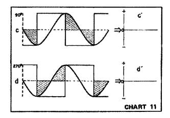
2-3. Potential at points (c) and (d) becomes that shown at a b c' and d' in the chart 10 and 11. Phase differences and output relations between pilot signal and detection signal are as shown in the following chart 12.
