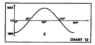
2-4. Since points @ and @ are connected to the differential amplifier, its operation creates the following relations. Let the potential at @ be E @, at @, E @ and at @, E @. Then E = K { E @ - E @ }. Furthermore K>0. The output potential at a undergoes the change shown in chart 12, also due to the phase difference between the pilot signal and detection signal j added to Tr3.
